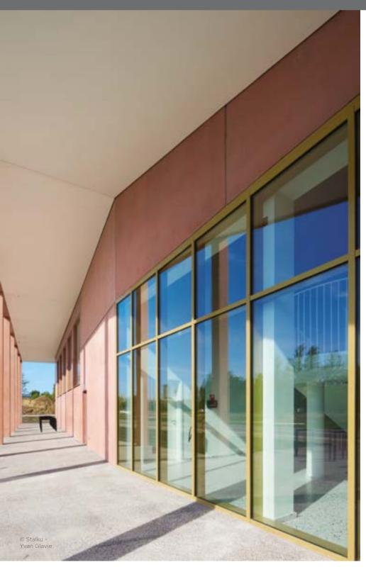
The **MC WALL** executed as a traditional curtain wall has a wide choice of clamp and cover profiles as an aesthetic finish. Style profiles are available up to a depth of 326 mm. Because we extrude at lengths of 7 metres as standard, a free span can be created in almost all situations without using a slide-in profile. A wide choice of profiles makes it possible to bring the posts and rails into one plane on the inside.
